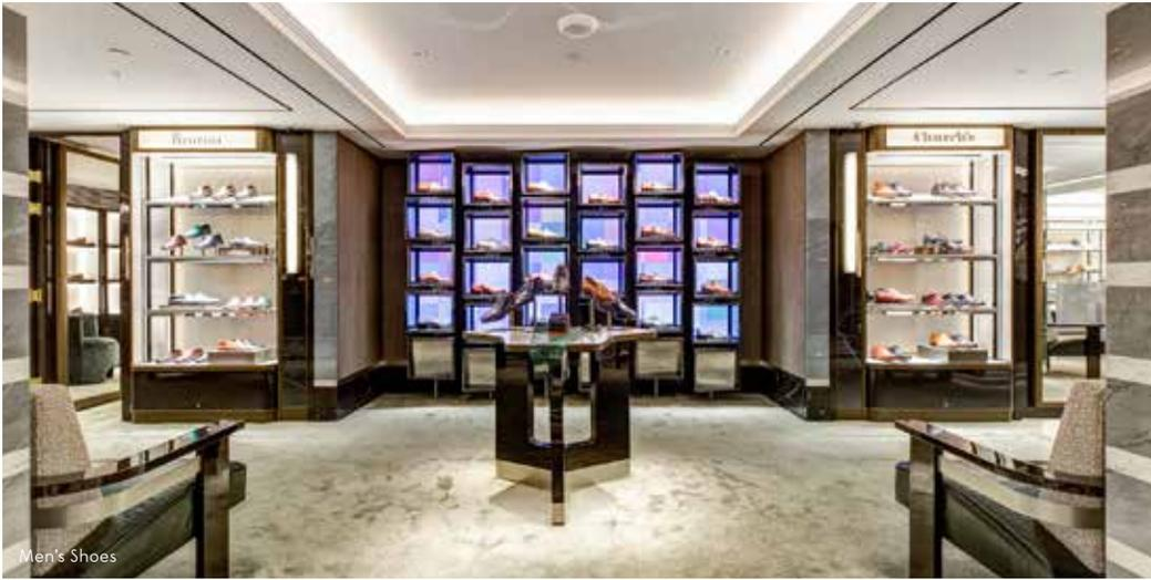
High-powered, individually-focused LEDs were used for each shelf, so every shoe is highlighted and uniquely lit. Two pop-up TV walls display a single shoe within a TV-like box which has a display monitor behind, forming part of a large bank of screens streaming custom content. These are located off the main central escalators and end walkway joining the three rooms, drawing customers in.
