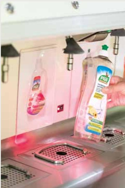
The refilling system recognises the product from the barcode on the bottle and fills it with the required quantity at the press of a button.
